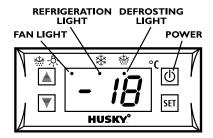
The thermostat has been pre-set, and in most cases it is not necessary to adjust the settings. When the appliance is operating normally, the display will show the current temperature. To display the set temperature press the strong button. Press the button again to return to normal operation.
