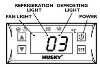
The thermostat has been pre-set, and in most cases it is not necessary to adjust the settings. When the appliance is operating normally, the display will show the current temperature. To display the set temperature press the s
